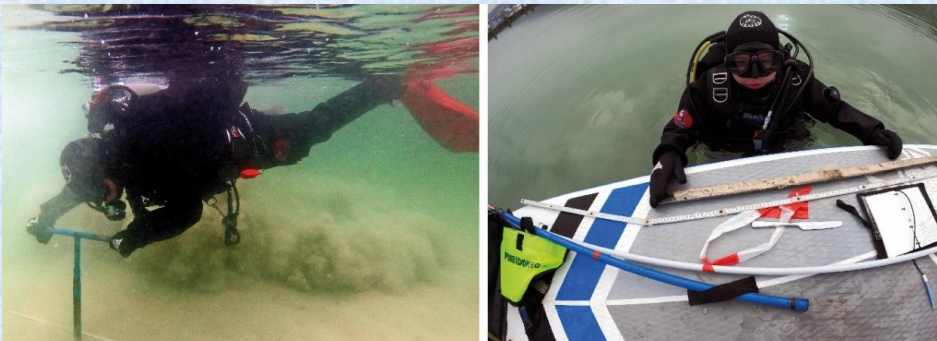
The prospection method of hand-operated sediment coring was applied by scientific divers
